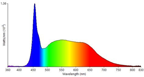
Testing was performed in accordance with LM-79-08.
